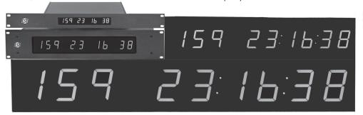
Each unit requires only a single pair of wires (although coax is recommended in certain environments) between itself and the Master Clock (or other source of time code). The wiring arrangement may be parallel, serial or both. Applications requiring extra long cable runs or signal isolation may require a Distribution Amplifier, refer to pages 22 & 23.
