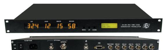
A nine-digit .56" amber LED display (Days, Hours, Minutes & Seconds) provides a readout of the input/ output time code. The IRIG time code input and outputs are via rear mounted BNC connectors. There are two outputs of the AM signal and two outputs of the TTL signal. The 1pps signal is also available on a pair of BNC connectors. The ES-295 is housed in a single height rack mount enclosure which is black anodized.
