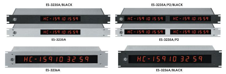
As the units read the event status codes, a minus sign is displayed indicating a countdown condition. During up-count conditions or while reading IRIG-B the minus sign is not displayed. Both units have two additional LEDs, one displays an alpha-numeric character (A-Z; 0-9) that provides a "project code" and the other digit displays the letter "H" to indicate a hold status in the "event countdown".
